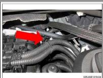
Visually inspect engine wiring harness and tank vent valve line.
