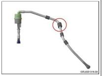
Install the new spacer after the bend between the first and second existing spacer on the tank vent valve (TEV).
