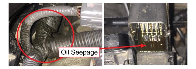
If related engine wiring harnesses and / or connectors are contaminated, the harness itself may also need to be replaced if degreasing affected components using a spray parts cleaner is unsuccessful.
