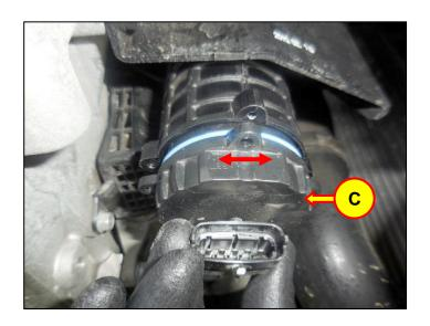
9. Slowly rotate the cap assembly (C) a half-turn clockwise to untwist the wires.
