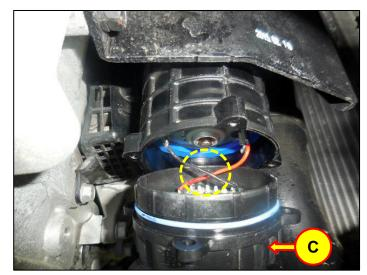
10. Disconnect the cap terminals using long nose pliers (D). Note the wire color installed at each terminal before removal.
