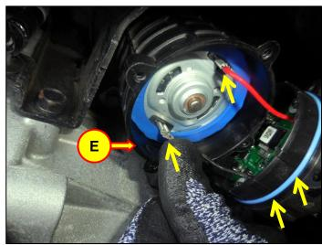
12. Slowly rotate the cap (F) a half-turn counterclockwise to cross the wires and push firmly until the cap is completely seated to the vacuum pump.
