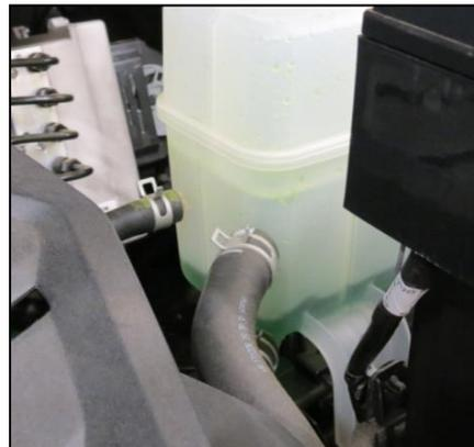
H-2. Using GDS with Ignition ON, perform the P/E cooling system air bleeding procedure.
