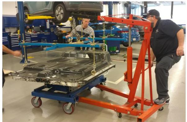
F-3. Install the replacement battery to the vehicle in reverse of the shop manual removal instructions.
