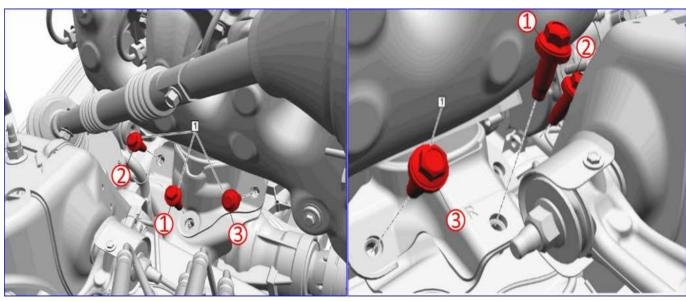
**Important:** Do Not use Impact wrenches when tightening the engine mount to frame bolts, or damage to threads in the frame may result.
