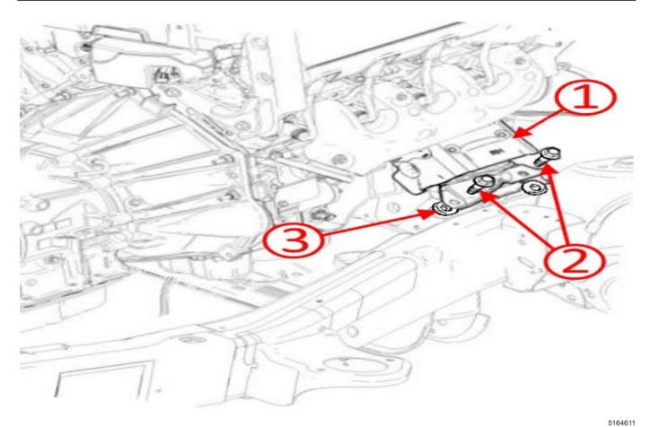
**Note:** Pause after loosening any of the mount bolts during these steps to determine the effect of the idle vibration on the Pico, at the seat track while making note of effect from each bolt location.
