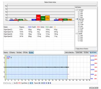
**Note:** Amplitude (mg) readings from a single-axis pico sensor will be approximately 10% lower than with a tri-axis sensor. For example a reading of 4 mg using a tri-axis sensor, would likely measure as about 3.6 mg on a single-axis sensor.
