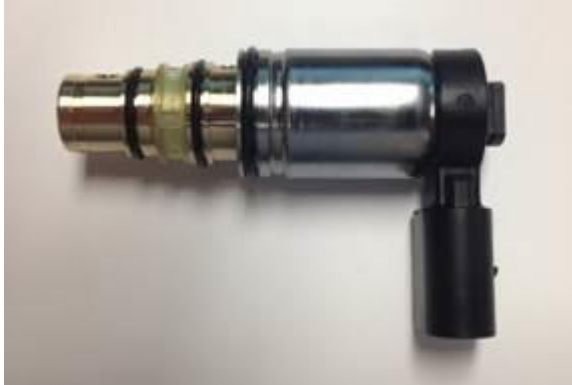
Figure 1 -N280- A/C Compressor Regulator Valve 1K0260839
