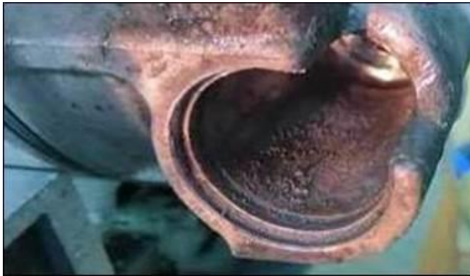
Figure 14. Corrosion in the -N280- A/C Compressor Regulator Valve bore.
