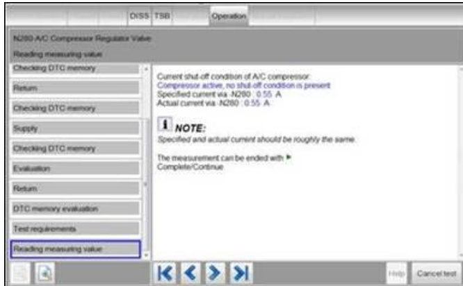
Figure 5. Checking N280 signal value Measuring Value Block.
