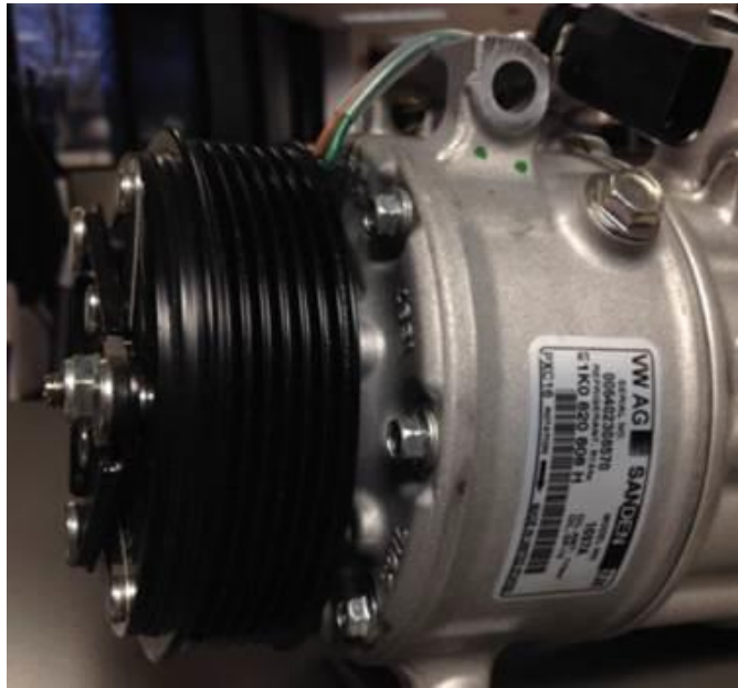
Figure 8. MY2016 AC compressor with clutch (Sanden)
