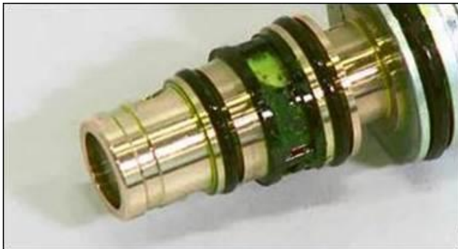
Figure 15: Severe contamination at the -N280- A/C Compressor Regulator Valve filter screen.
