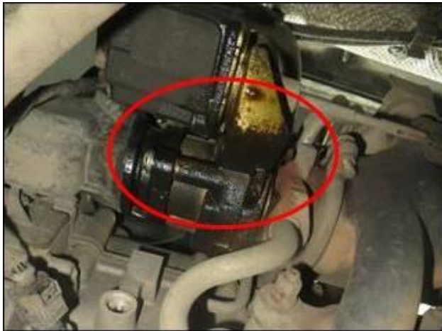
Figure 1: Example of engine oil at the Turbocharger Air Intake Hose.
