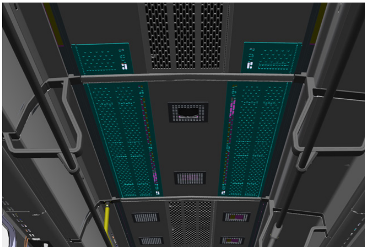
Figure 3 - Typical Location of Return Air Grill
