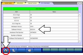
d. If the Software Version listed is **not** at the latest level (shown in the "BMU/Sub-BMU Reprogramming Chart" in this TSB), proceed with the next step. Click the Home button to return to the System Select screen.
