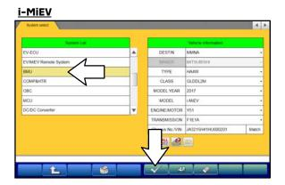
Select BMU" (for i-MiEV) or "BMU(SUB)" (for Outlander PHEV)" from the System List, then click on the check mark at the bottom of the screen.
