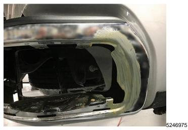
5. Using a bristle type paint brush, apply one even coat of the wax on the left and right side of the rear bumper as shown.
