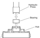
Install the new bearing using an arbor press fitted with a hollow or stepped punch face to press only on the outer housing of the bearing. Failure to follow procedure will
