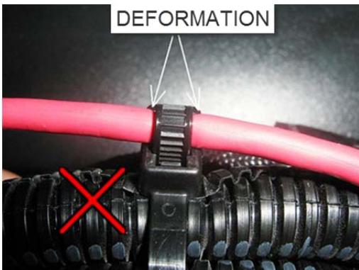
Cable tie tighten in excess on the LTD. Tighten cable tie on LTD by hand only. Tighten just enough to prevent LTD from slipping from one side to the other inside the cable tie loop
