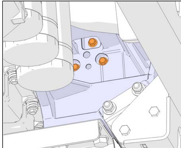
FIGURE 45: IDLER / TENSIONER ASSEMBLY MOUNTING SCREWS
