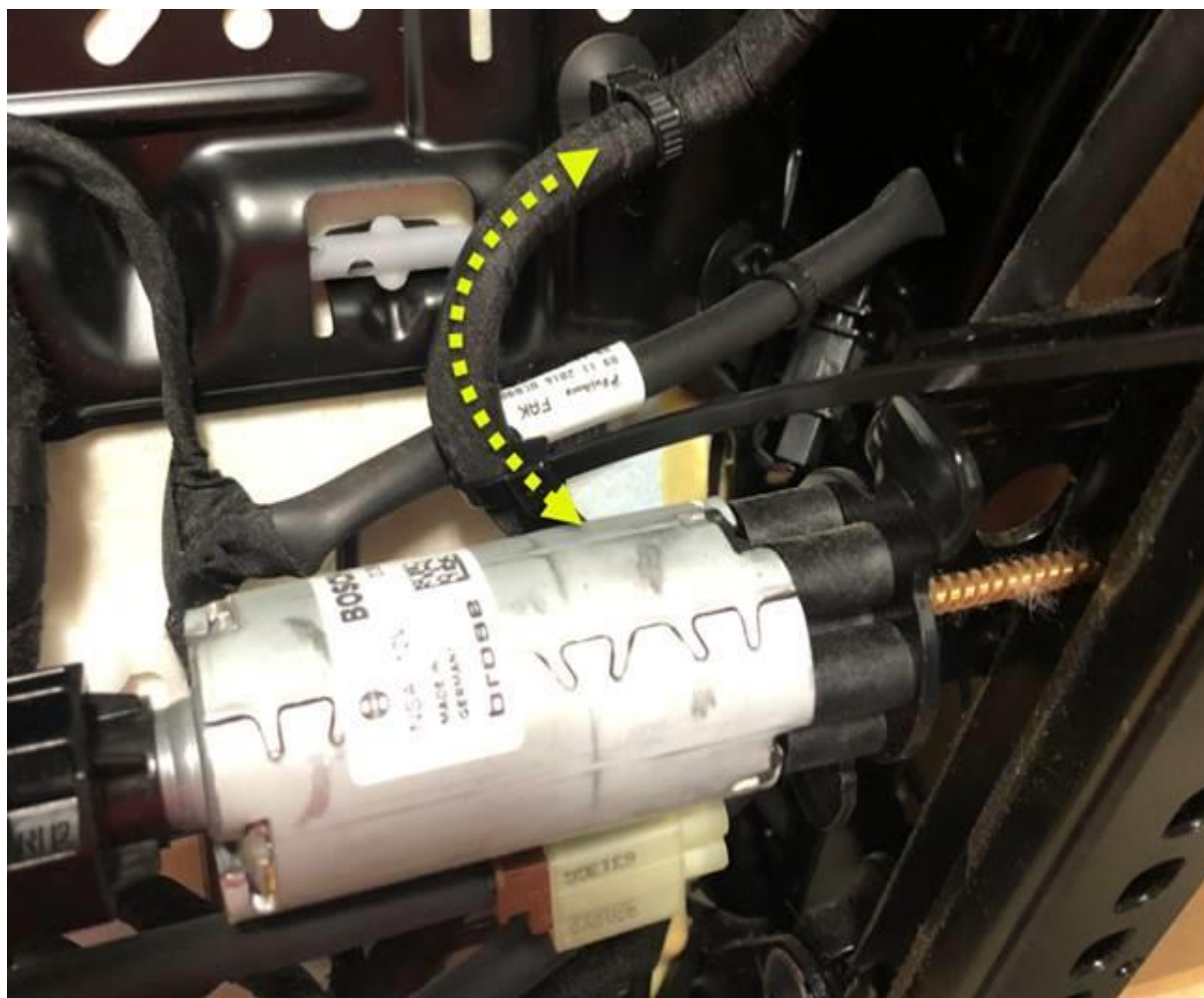
Figure 3. Attach the second cable tie to the yellow marked area.
