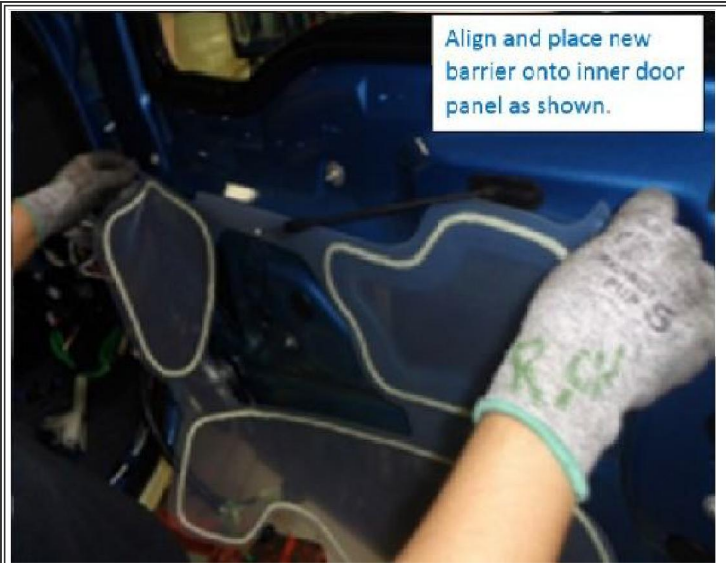
Figure 4: Plastic Vapor Barrier aligned and in place.
