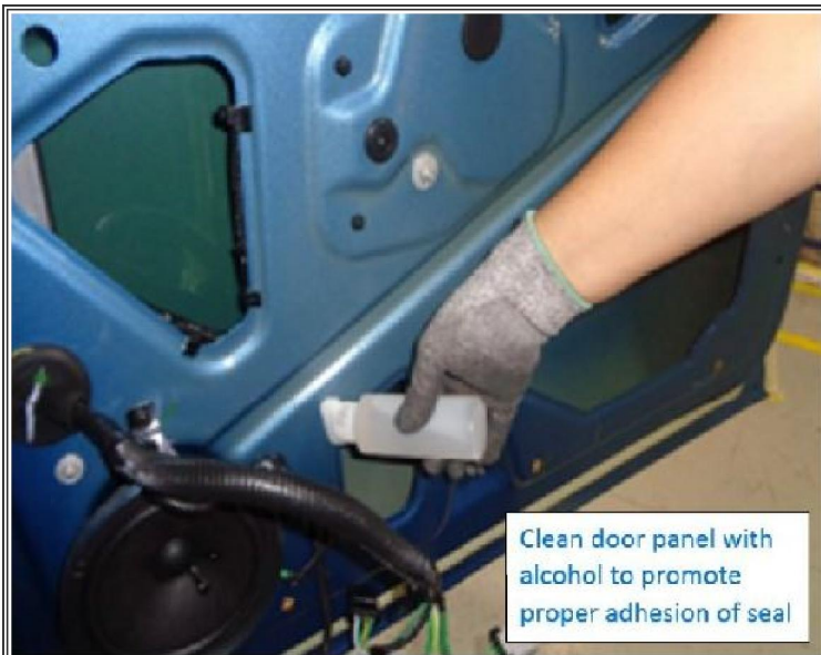
Figure 2: Cleaning the Door Panel of Old Residue
