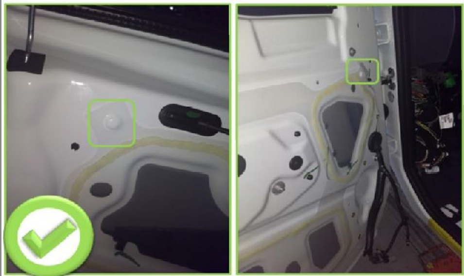
Figure 3: Door Alignment Features for Placing Barrier Sheet in proper location.
