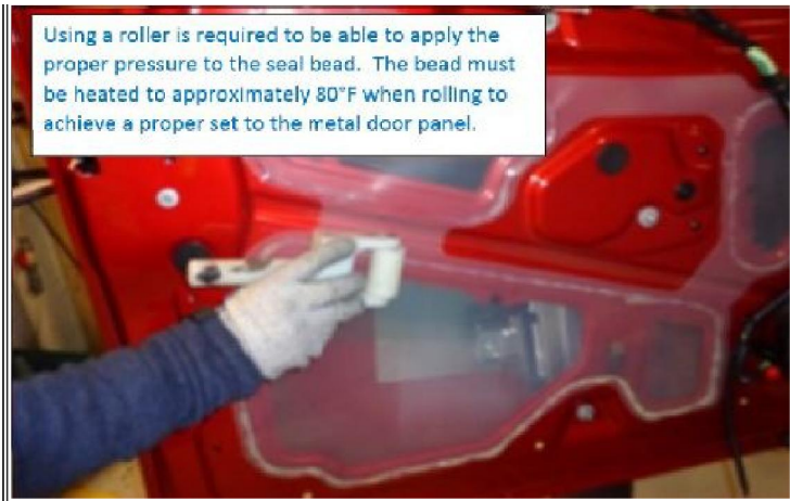
Figure 5: Rolling new sealant to door panel for proper adhesion
