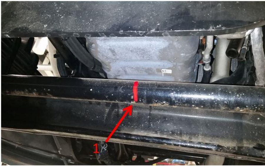
Figure 1: Tie rod assembly
