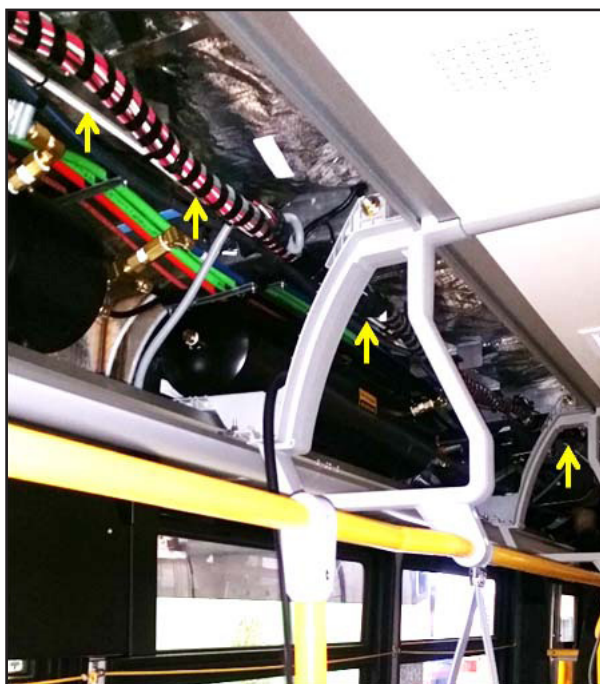
Figure 22 - Front-to-Back Cable Routing
