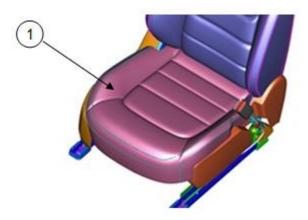
**NOTE:** It is not necessary to completely remove the side seat covers. Loosen the front of the covers only (as shown below) to access the side of the seat cushion.
