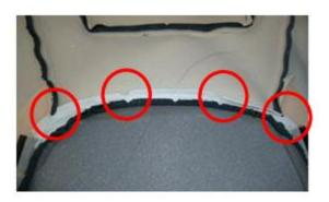
c. Adjust the wire position so that it is even on both sides.
