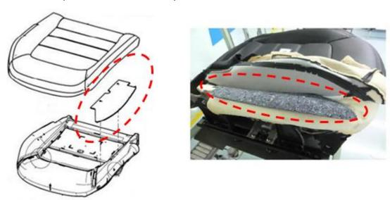
b. Place the felt pad onto the new seat cushion pad and tie the seat cushion pad, felt pad and seat cushion trim with two (2) hog-rings.
