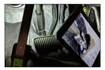
6. If the intermediate steering shaft universal "joint bottom to floor panel" measurement is within specification and witness mark is present, or witness mark was missing and universal joint bolt was torqued to specification, then install all removed parts in the reverse order of removal. The action is complete.
