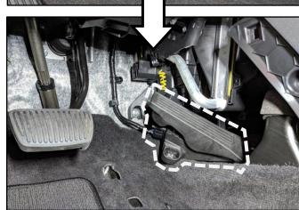
2. Roll the carpet back to expose the intermediate steering shaft universal joint.
