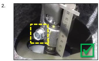
If no mark is present as shown, verify that the bolt is torqued to 23.9 - 27.5 ft-lb (32.4 - 37.3 N.m, 3.3 - 3.8 Kgf.m.) and open a techline case.
