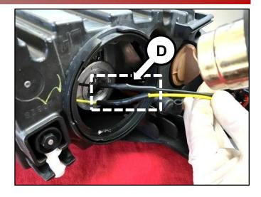
Install the new connector (E) to the low beam bulb.
