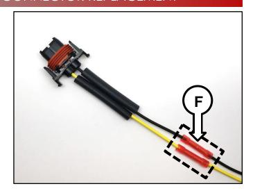
Crimp the butt splice connectors at two
