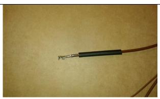
8. Slip shrink tubing (Part# 61 13 1 379 833) over wire of ground cable (Part# 61 12 7 492 553) containing crimp connector (as shown).
