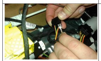
4. Open connector and pull out brown ground cable, pin 8.
