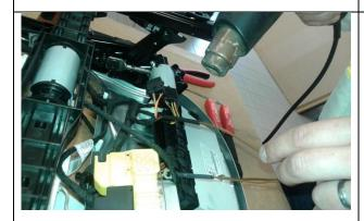
10. Reposition shrink tube over connection and heat.
