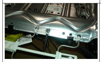
14. Attach eyelet wire from Ground cable at drilled hole with (4.8mm X 9mm) rivet (part# 07 14 7 444 158).
