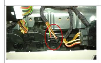
3. Remove connector A245\*3B from the seat module.
