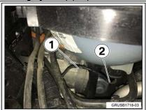
Once the expansion tank is removed, Remove the protective tape (1) approximately 4 inches away from the connector and cut the connector off the harness (2)
