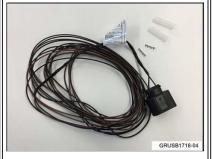
The repair harness (PN 61 11 9 312 324) comes with two spice terminals and two heat shrink sections.
