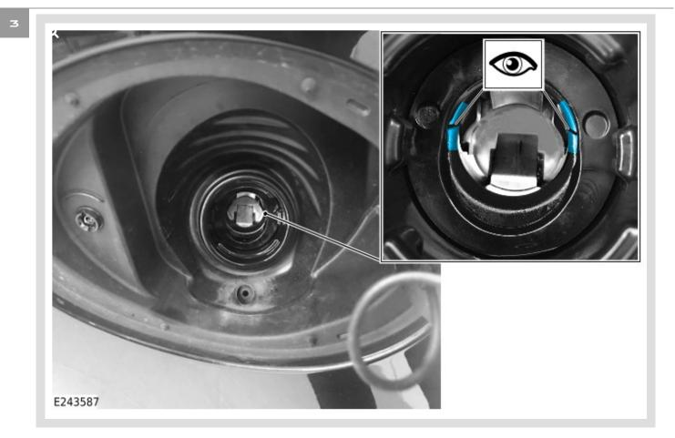
Inspect the fuel filler neck for signs of cracking as shown.
