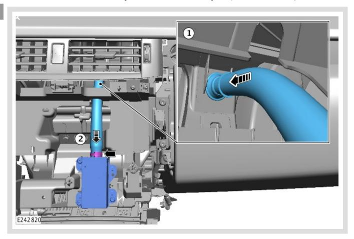
Install the new air ionizer hose.
