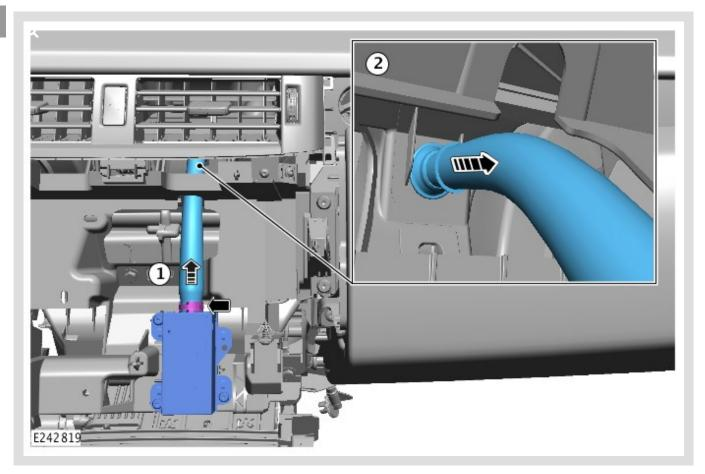
Remove the air ionizer hose.
