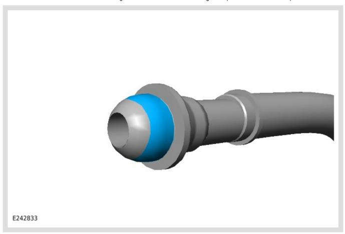
Apply a small amount of grease (PEOX612 or equivalent) as shown to the outside of the new air ionizer hose.
