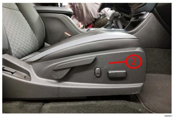
The graphic examples above shows the different thickness adjustments and controls between the driver seat cushion (1) and the passenger seat cushion (2).
