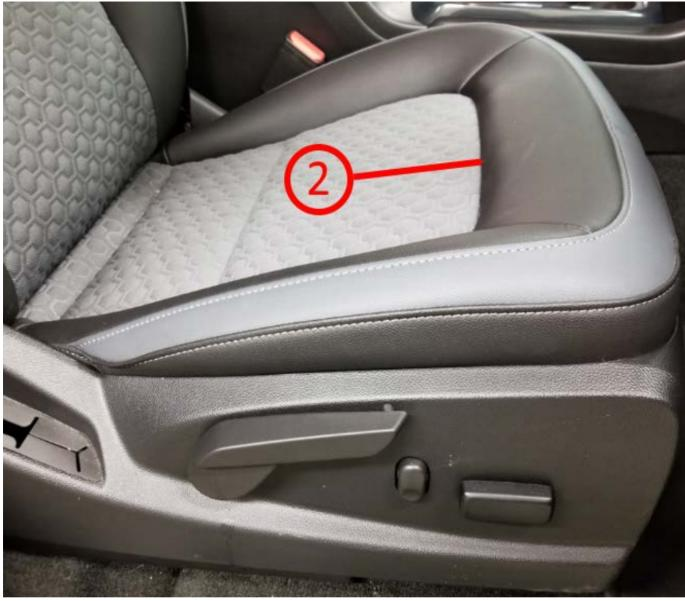
The graphic examples above shows the different thickness in the bolster area between the driver seat cushion (1) and the passenger seat cushion (2).
