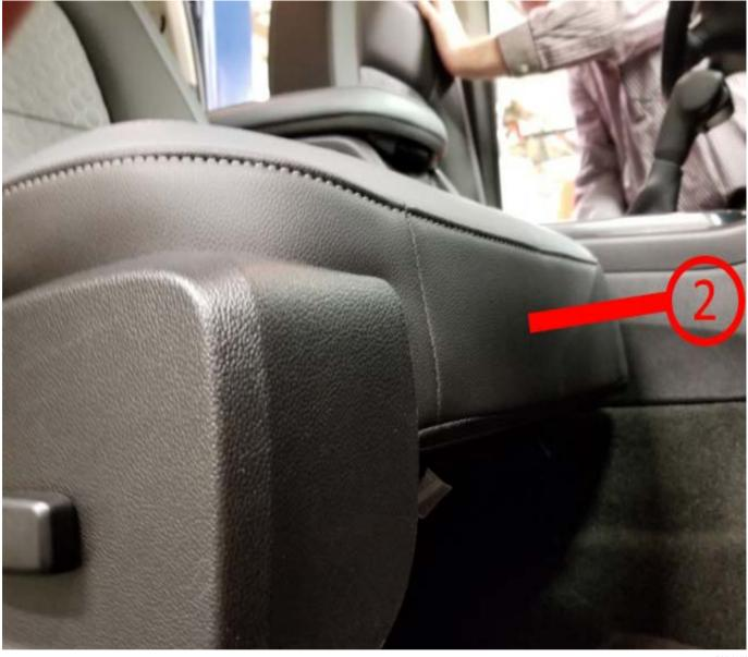
The graphic examples above shows the different appearance in thickness of the driver seat cushion (1) and the passenger seat cushion (2).
