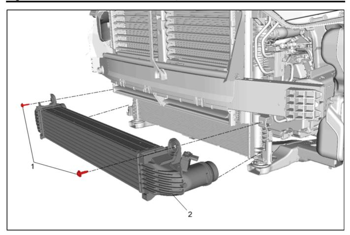
**Important:** The newly designed charge air cooler is wider and is NOT compatible with the existing lower baffle on the vehicle. The baffle will need to be replaced to accommodate the larger charge air cooler.
