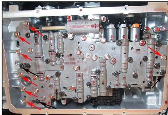
8. Remove 9 bolts and remove the E-module.
