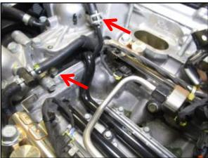
4 Push the pipe toward the rear of the engine and disconnect the forward end of the pipe from the housing.
