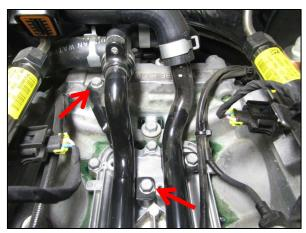
Remove the bolt near the front of the engine.Disconnect the clamp and hose.
