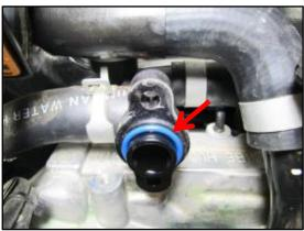
7. Install a new O-ring (part number 25462-3F300) on the end of the pipe near the radiator.
