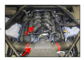
**2.** Remove the 2 bolts to the brackets that secure the pipe near the rear of the engine.
