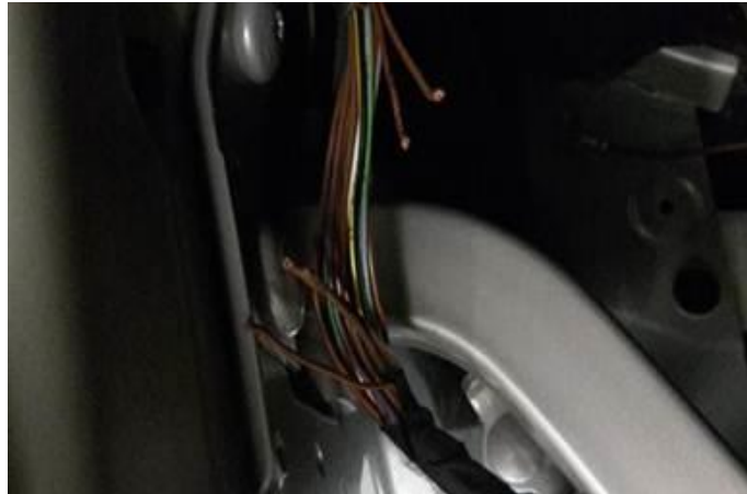
Figure 1. Wire damage at trunk hinge.
