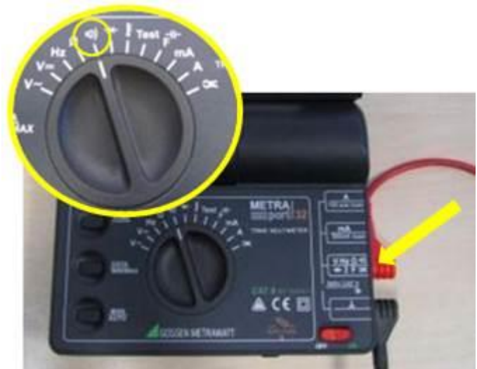
Figure 16. Set the VAG 1526 C to current flow check and connect the probe cables.
