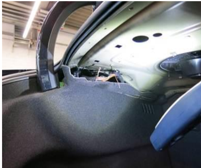
Figure 2. Wire damage at trunk hinge.
