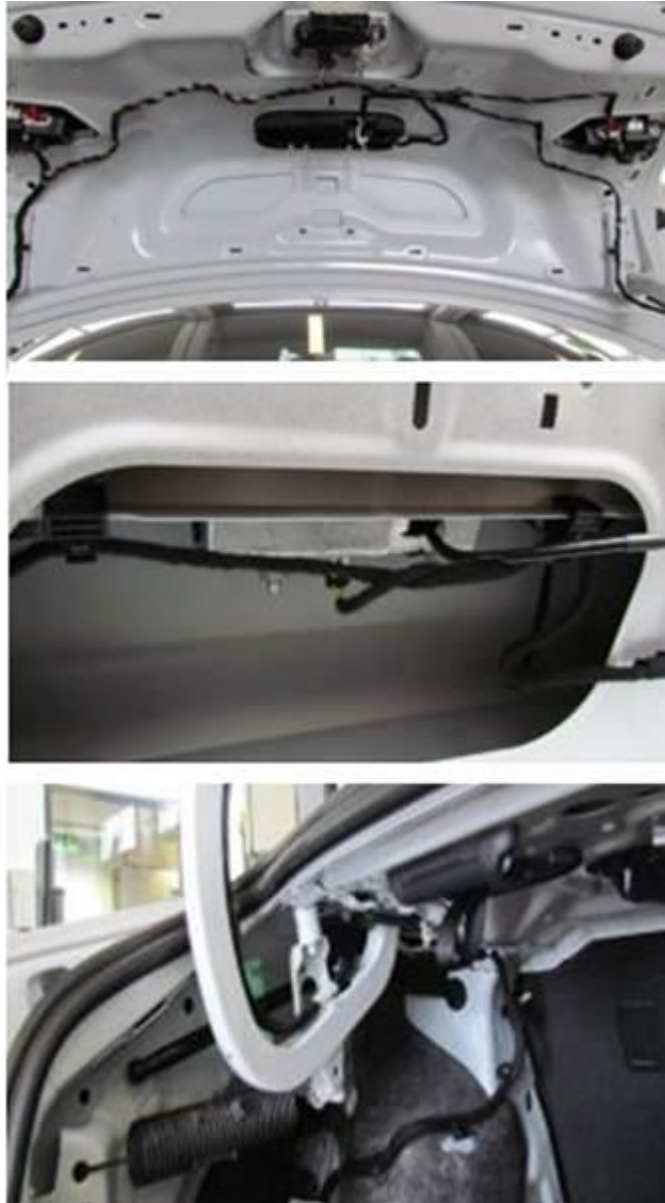
Figure 12. Examples of photographs of the routing of the wiring harness. The routing may differ depending on the vehicle.
