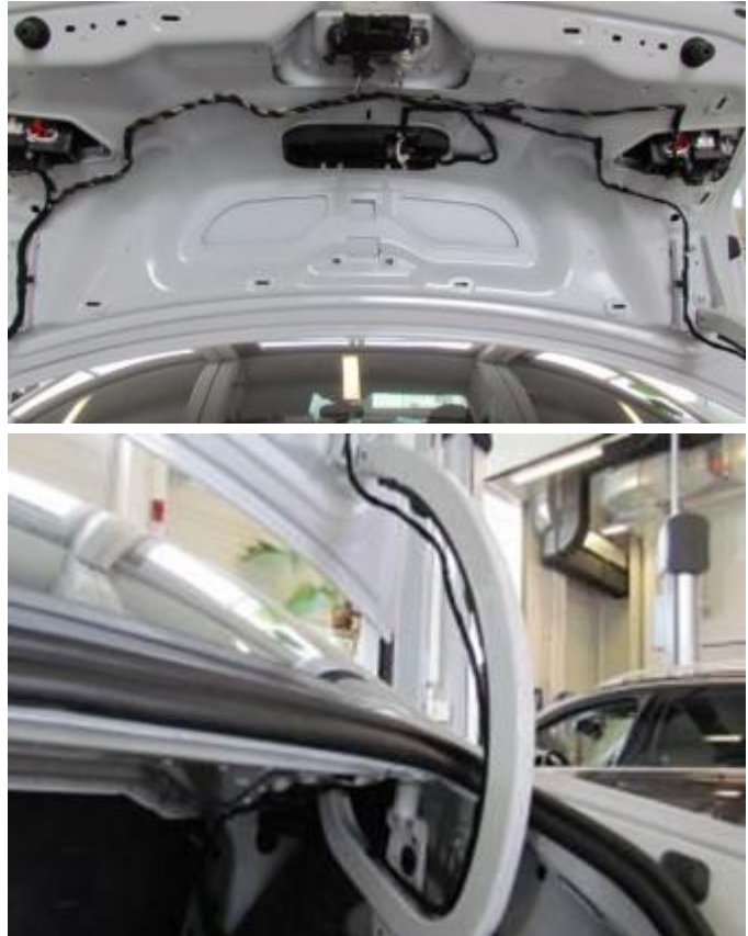
Figure 4. Examples of photographs of the routing of the wiring harness. The routing may differ depending on the vehicle.
