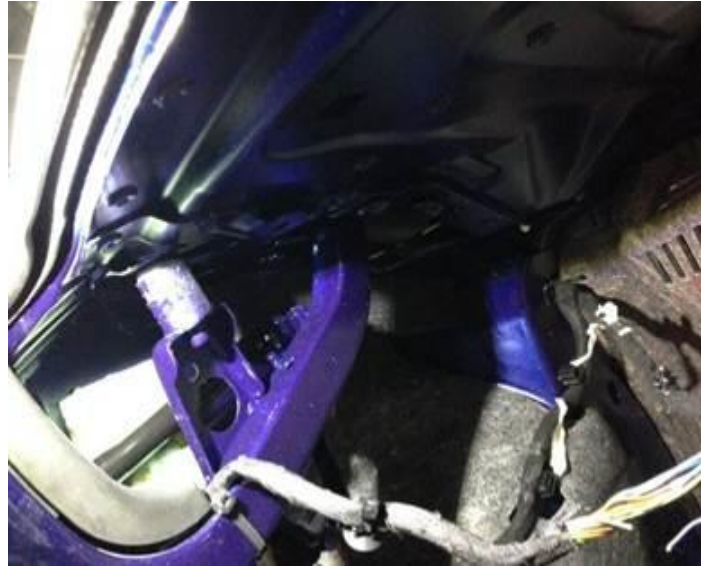
Figure 3. Incorrect wire routing at trunk hinge.
