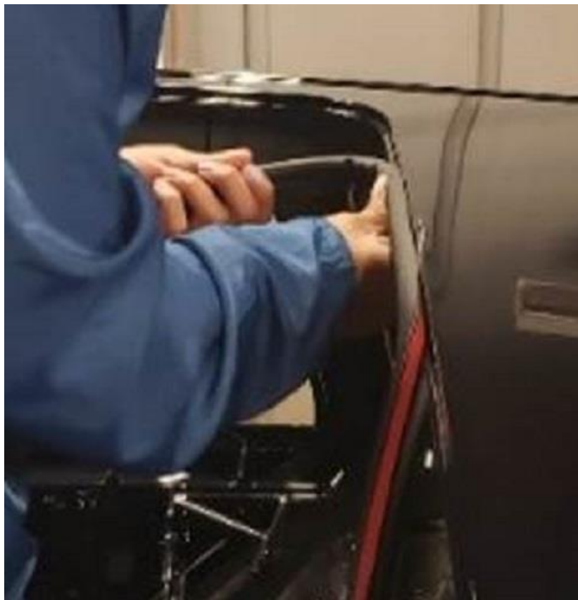
Figure 5: Example of installing the body side seal WITHOUT removing the “red” protective tape.
