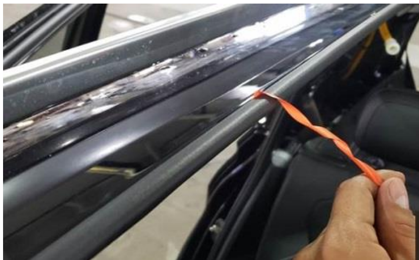
Figure 6: Example of removing the “red” protective tape after seal has been properly seated.
