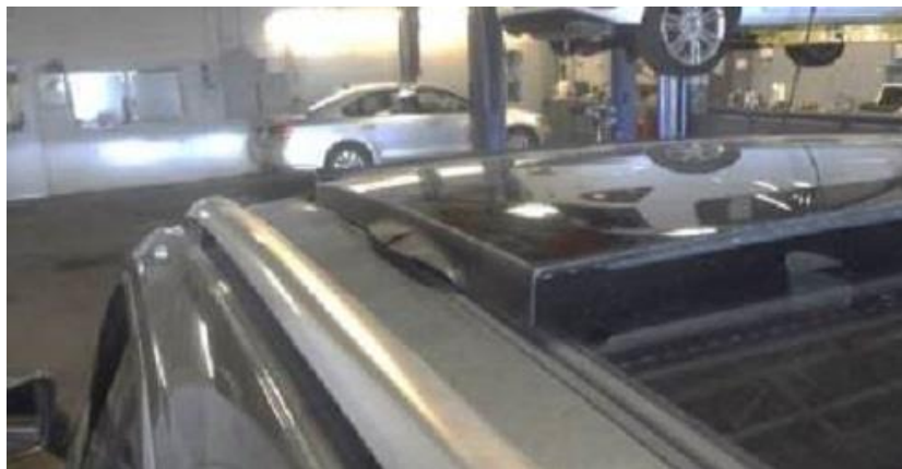
Figure 3: Example of the sunroof panel molded seal warped/deformation.
