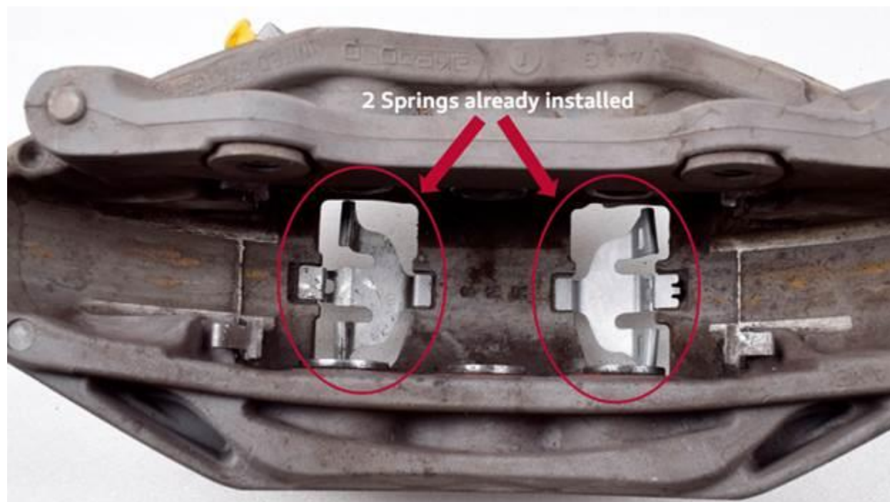
Figure 3. Spring configuration, after installation.
