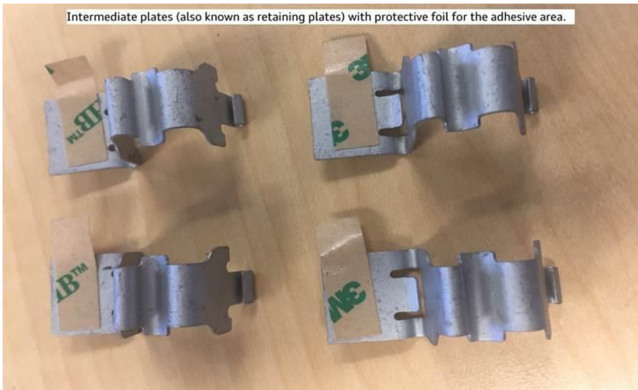
Figure 6. Intermediate plates (also known as retaining plates).
