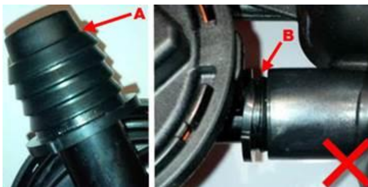
Figure 7. Plastic port extending past the grommet (A) causing installation issues (B).
