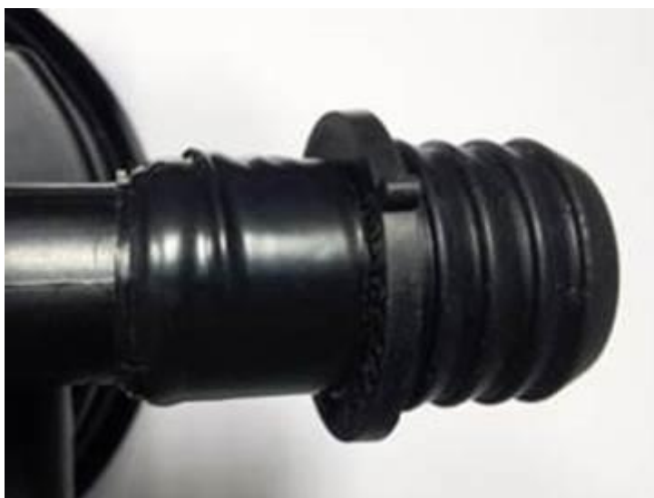
Figure 4. Vinyl layer supporting grommet.
