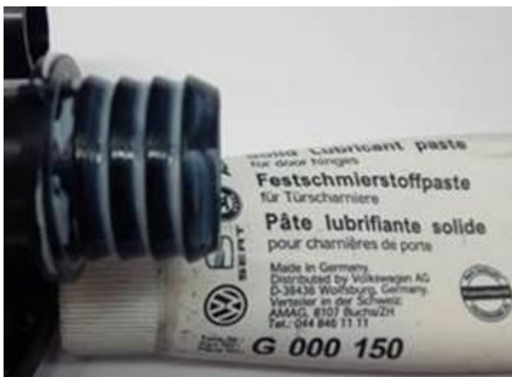
Figure 5. Grease film on the outer surface of the grommet.
