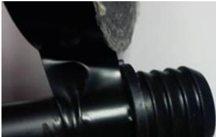
Figure 3. Wrapping vinyl tape behind the grommet.
