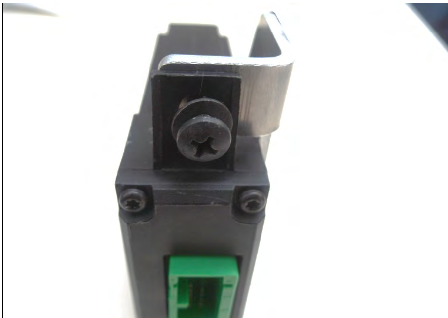
GATEWAY MODULE ON BRACKET – USE FLAT WASHERS
