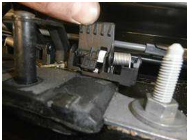
Figure 3. Debris in the rear lid closed sensor.
