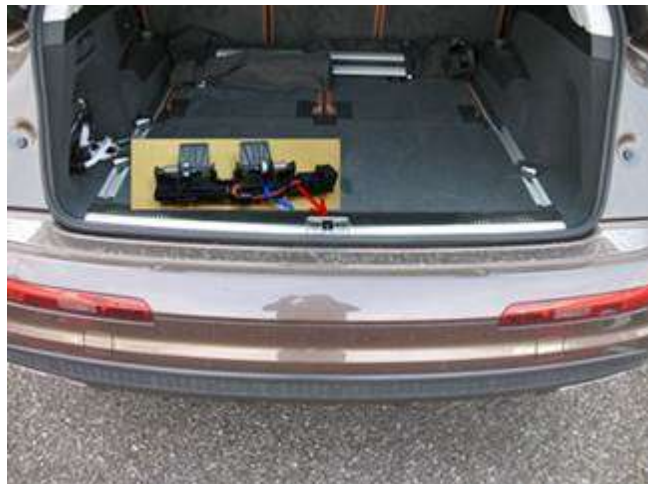
Figure 2. Rear lid closed sensor.
