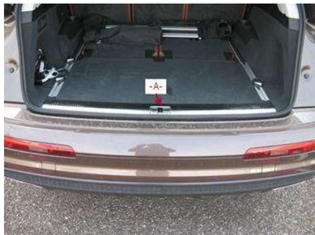
Figure 4. Striker cover opening.
