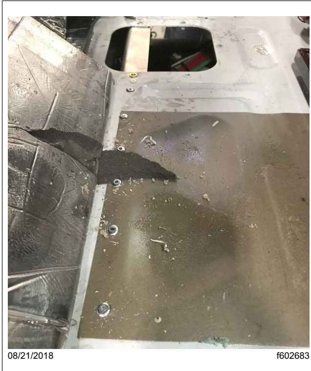
Fig. 5, Floor Support Riveted to the Cab Floor
