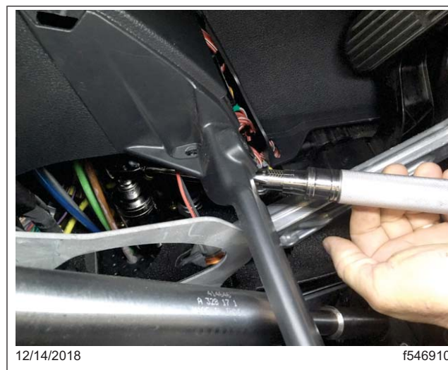
Fig. 3, Tightening the Brake Light Pressure Switch
