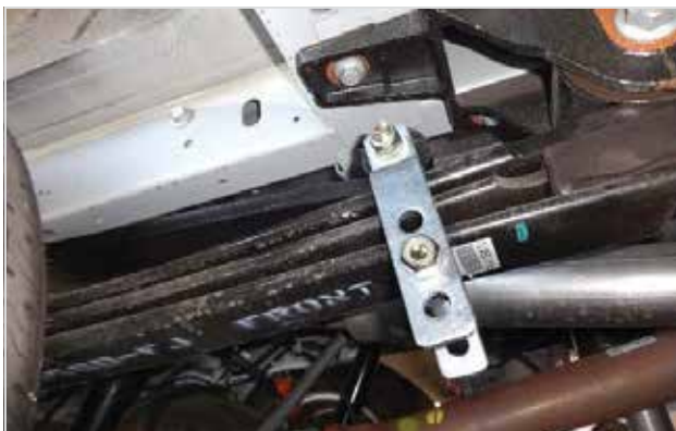
FRONT SUPERSPRINGS SHACKLE IN CORRECT POSITION
