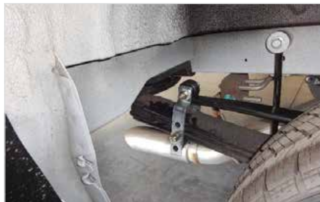
REAR SUPERSPRINGS SHACKLE IN CORRECT POSITION
