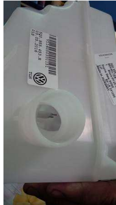
Figure 2. Windshield washer level sensor probes as viewed through the tank opening.
