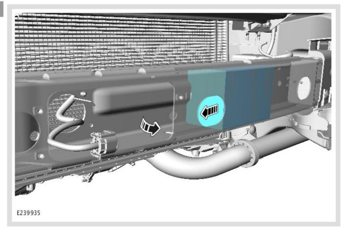
Only if necessary: remove and discard the existing foam block(s).
