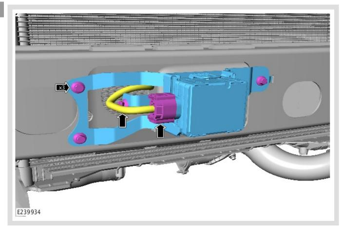
Remove the radar bracket.
