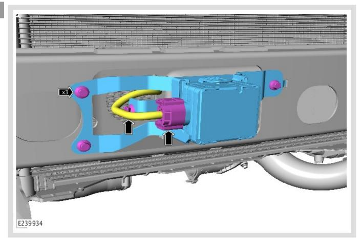
Install the radar bracket.
