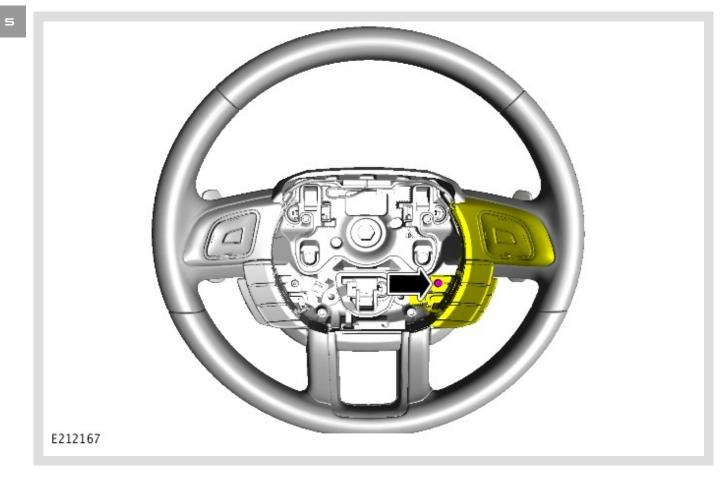
Remove the steering wheel right control switch fixing and position the steering wheel right control switch to the side.
