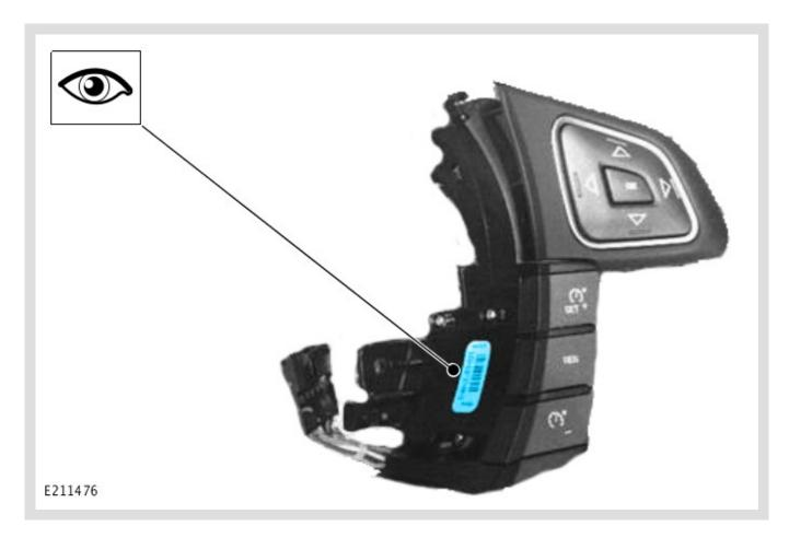
Confirm the part number (on the label) of the existing steering wheel right control switch.
