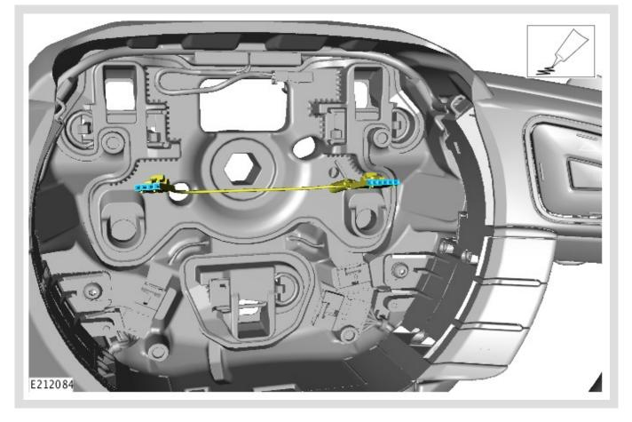
Apply the Nyogel to the front of the steering wheel left control switch lower electrical connector and the front of the steering wheel right control switch lower electrical connector.
