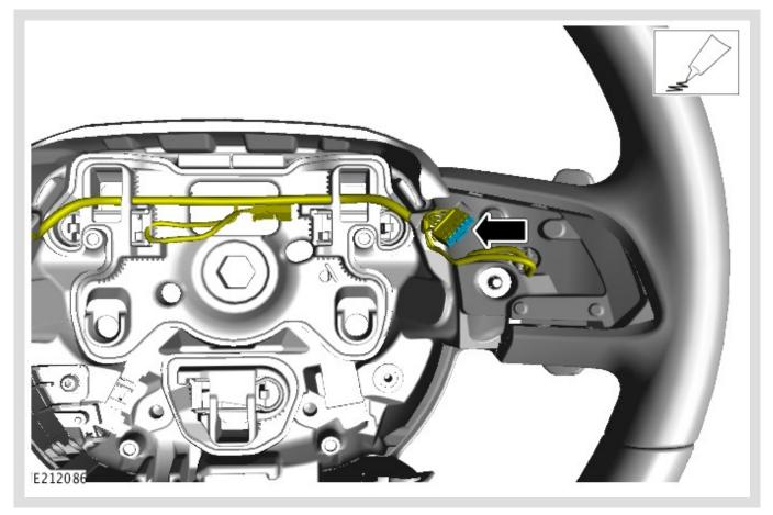
Apply the Nyogel to the front of the steering wheel right control switch upper electrical connector.
