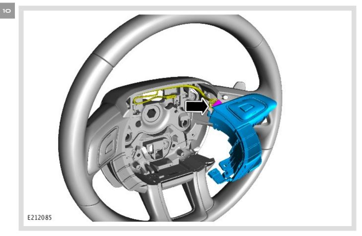
Connect the steering wheel right control switch upper electrical connector to the new steering wheel right control switch.
