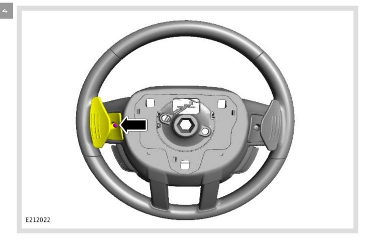
Remove the right paddle shifter fastener and position the right paddle shifter to one side. Do not disconnect the paddle shifter electrical connector.
