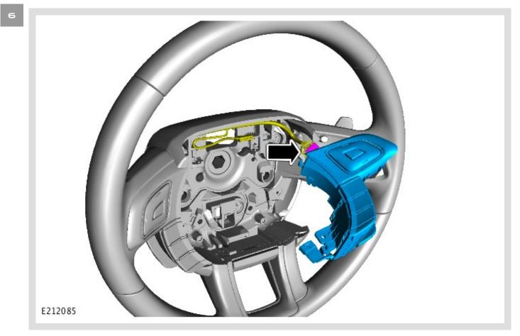
Disconnect the steering wheel right control switch upper electrical connector.
