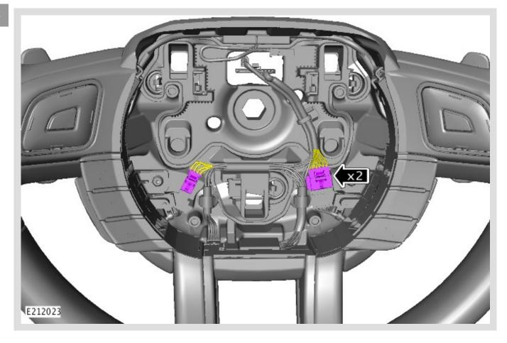
Disconnect the steering wheel right control switch lower electrical connector and the steering wheel left control switch lower electrical connector.
