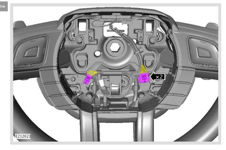
Connect the steering wheel right control switch electrical connector and the steering wheel left control switch electrical connector.
