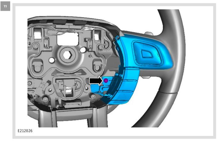
Install the new steering wheel right control switch.
