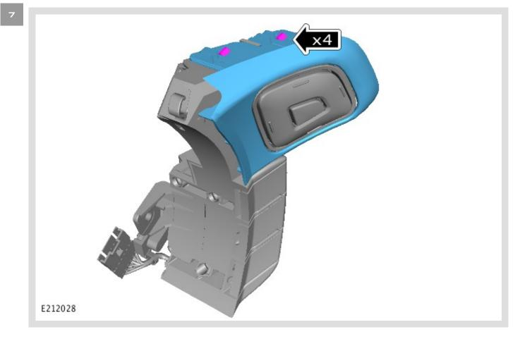
Remove the bezel trim from the existing steering wheel right control switch.
