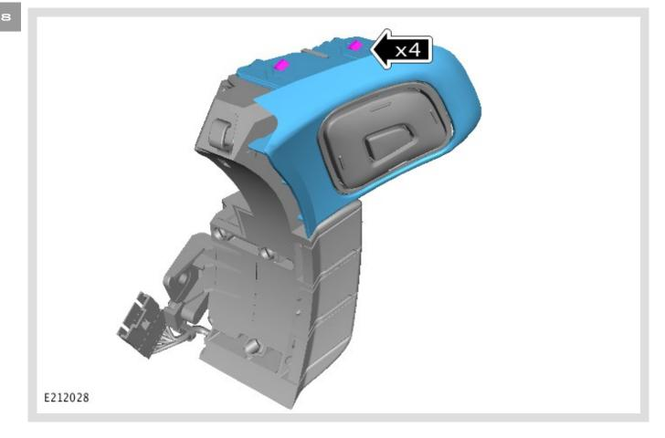
Install the existing bezel trim to the new steering wheel right control switch.
