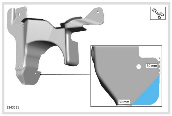
Using the measurements shown, remove the highlighted section of the front wheel arch liner center section.
