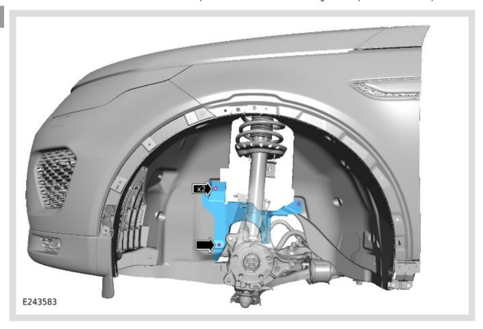
Use the enlarged hole (Step 4) and install the front wheel arch liner center section into the most upward position possible.
