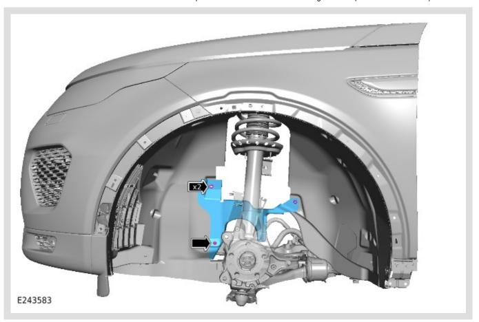
Remove the front wheel arch liner center section.
