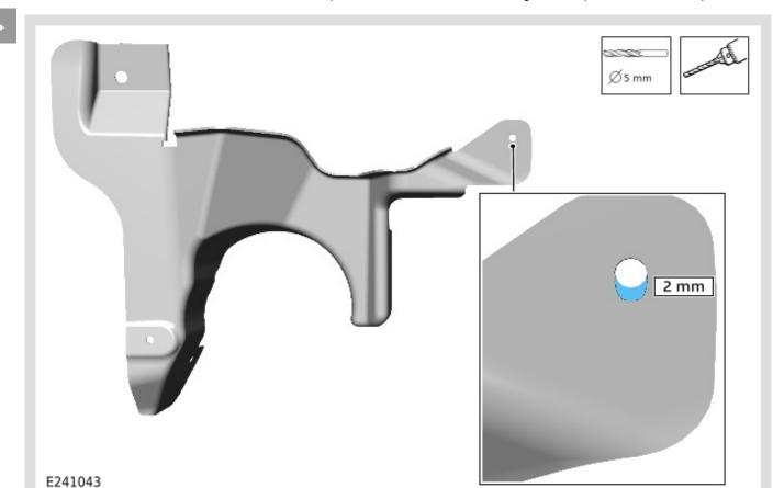
Use a suitable drill and 5 mm drill bit to enlarge the fastener hole downward by 2 mm.
