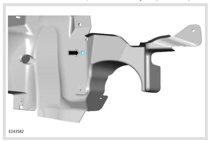
The front height sensor wiring harness must be installed as shown. Position the wiring harness fastening clip as necessary to the wiring harness.
