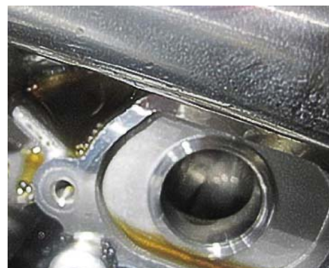
Fault type 1: Valve lift adjustment solenoid hydraulic leaking
