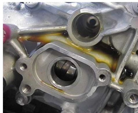
Fault type 2: Cylinder head cover leaking
