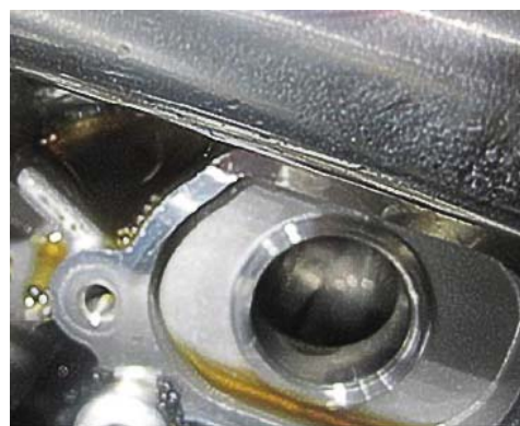
Fault type 1: Valve lift adjustment solenoid hydraulic valve leaking
