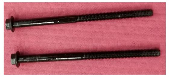
Calllout 3: Item 377 in SI document 4970174 (Qty1) replacement not required unless removed. Bolt is not typically removed during valve body replacement.
