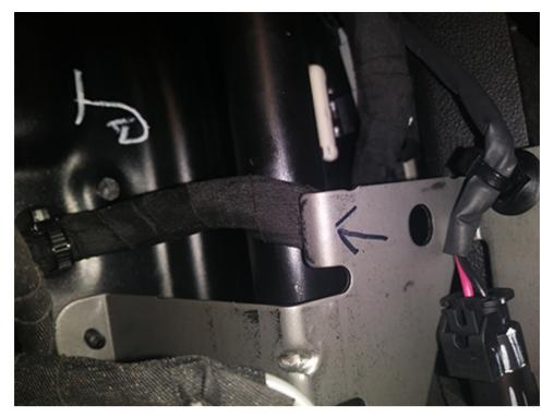
Repair or replace the seat harness as needed and re-route it so that it will not become pinched or damaged.
