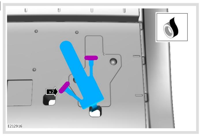
Install the anti-trap sensor using appropriate double-sided tape under the locating tabs as shown.
