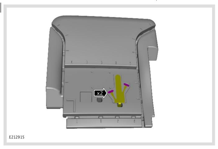
Release the 2 anti-trap sensor locating tabs from the seat cushion.
