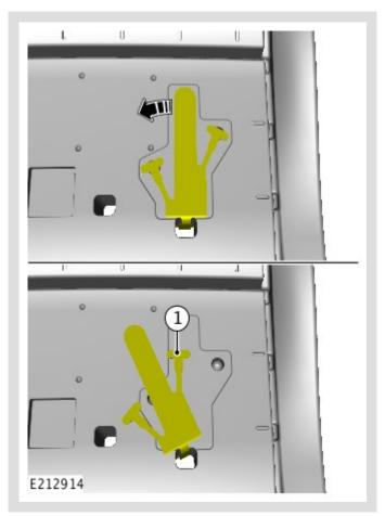
Position the anti-trap sensor so that locating tab (1) is oriented as shown.
