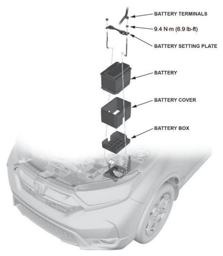
7. Install the parts in the reverse order of removal.
