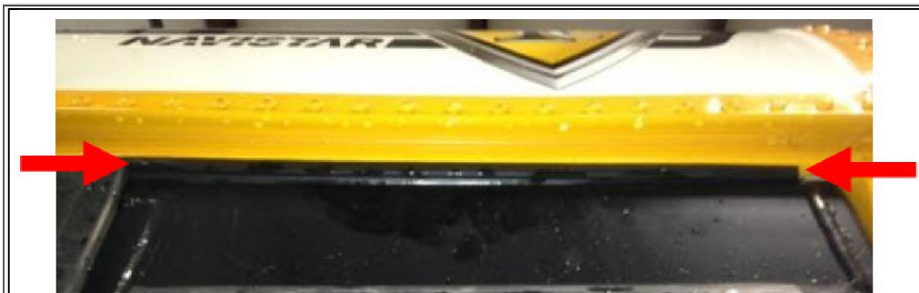
Upper Door Casing Seal Evenly Compressed
