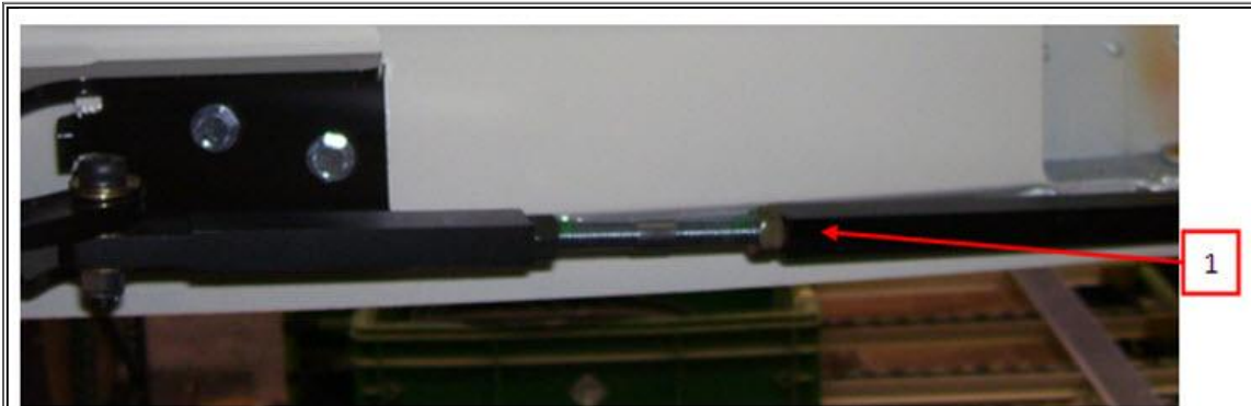
1. Tie-Bar Assembly (Aft Shown)
