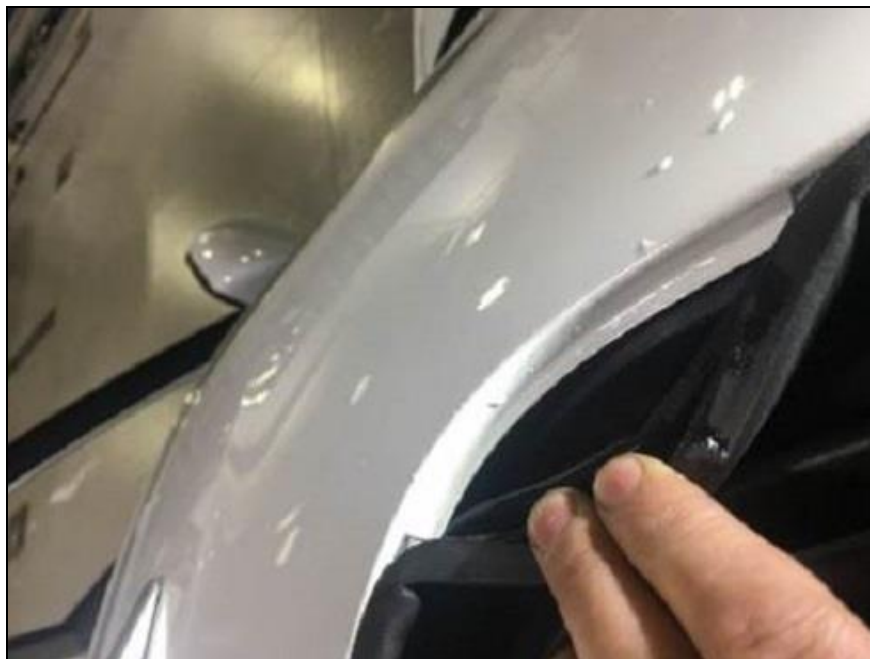
Figure 2: Example of the sunroof body side seal not having proper adhesion to the body.
