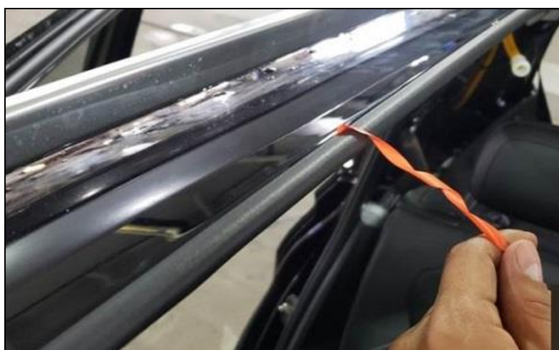
Figure 6: Example of removing the “red” protective tape after seal has been properly seated.
